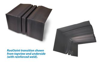
The upper flange counterflashes the termination bar and underlying membrane ensuring that penetrations made by the attachment of the termination bar are completely sealed. The upper flange is further flashed to the roofing membrane by means of the roofing manufacturers' standard flashing tape or by over-welding a strip of roofing.
