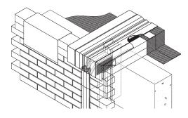
Like the solid-wall closure, the cavity-wall RoofJoint closure, is a factory-fabricated transition piece made from Seismic Colorseal. The difference is an extended, horizontal setback portion of coated foam to bridge the cavity from facade to structural backup wall. The sides of the "bridge" are additionally coated with silicone to seal them against moisture in the cavity and to constrain the
