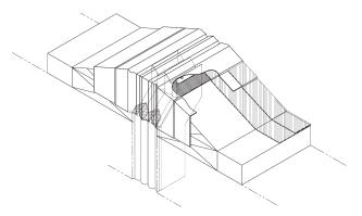
This single unit piece has factory-coated silicone bellows on the top and upper-back faces for integration with Seismic Colorseal in the wall and Horizontal Colorseal as a secondary seal and insulator across the roof. The silicone-coated top side of the closure is shaped to match the underside of the RoofJoint extrusion.
